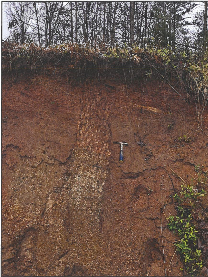
Figure 4. Exposed stratigraphic profile of weathered bedrock surface soil in the vicinity of where the transmission line crosses Hogan Creek (facing east).
