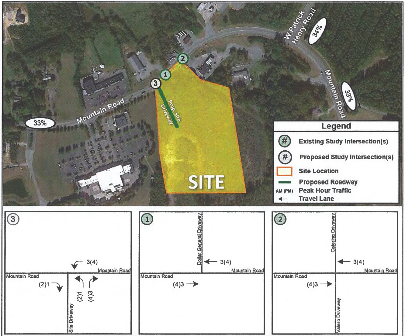
Figure 6: Site Trip Distribution and Assignment
