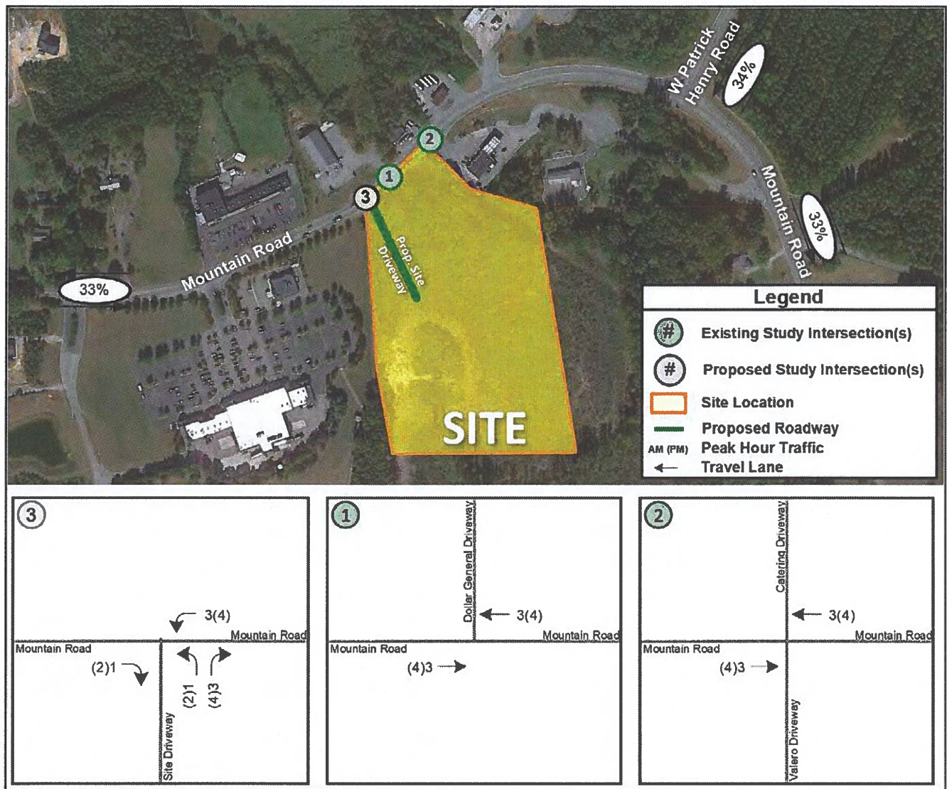
Figure 6: Site Trip Distribution and Assignment
